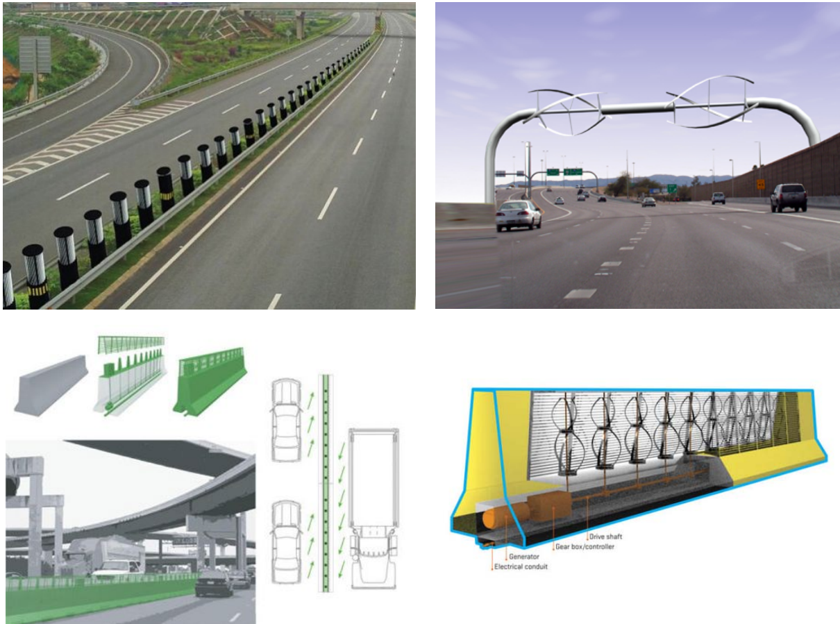
Figure 12: Examples of Wind Generation Systems that Use Air Movement from Passing Traffic to Produce Energy 79
