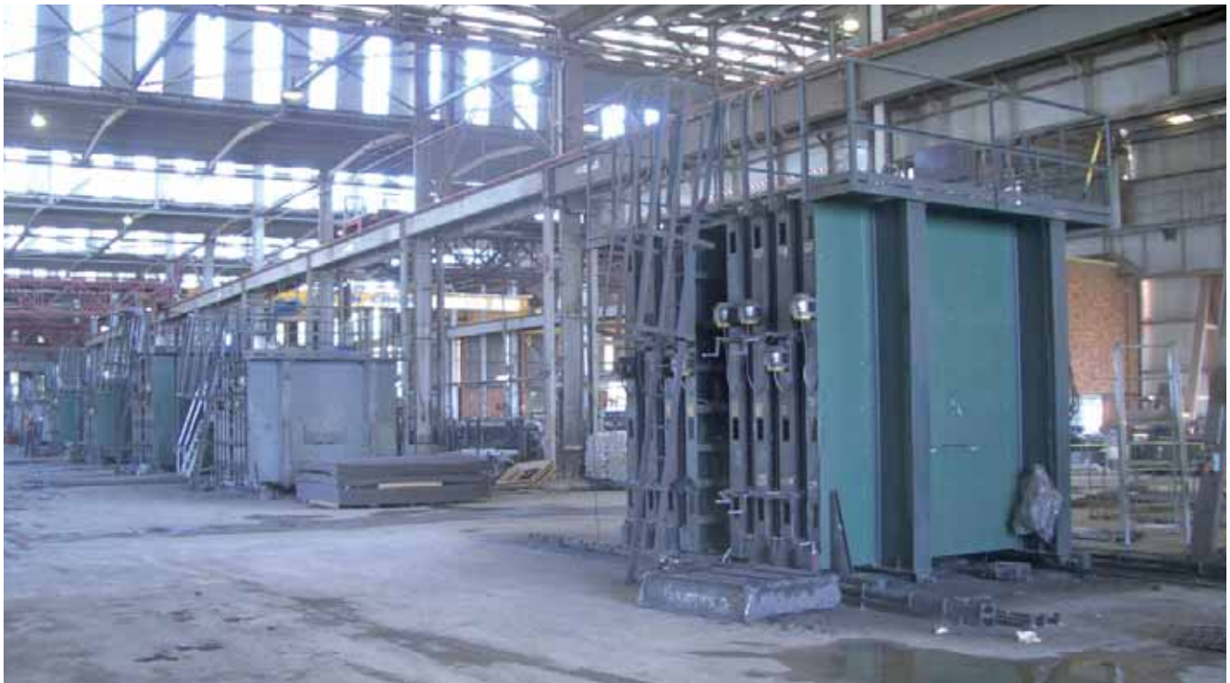
Vertical sound barrier moulds (battery moulds)
