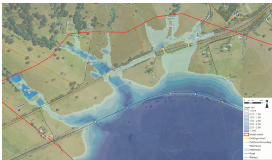
Figure 2. 100 year flood simulation without preventative works Source: NSW RMS
