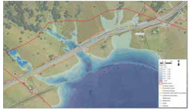
Figure 3. 100 year flood simulation after preventative works Source: NSW RMS
